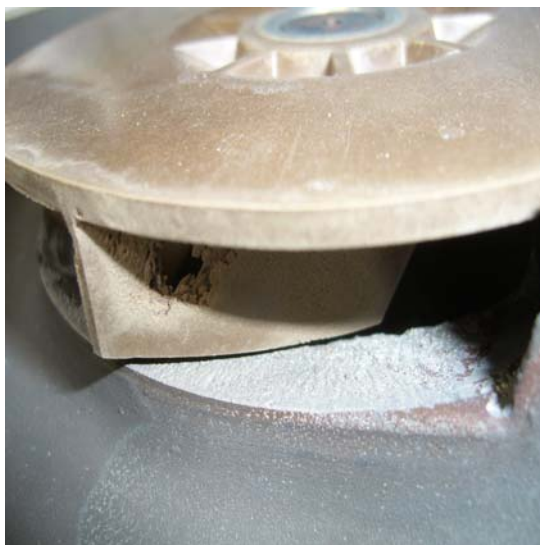
A 14 Flywheel of the coolant pump, cavitated
