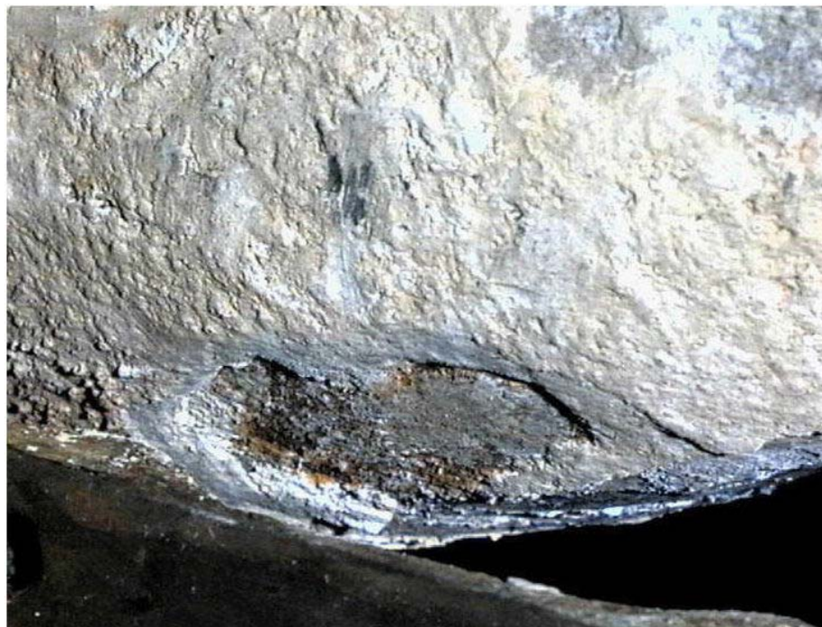
A 12 Limescale deposits on a cylinder liner
