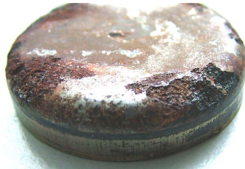
A 10 Sealing cover, corroded
