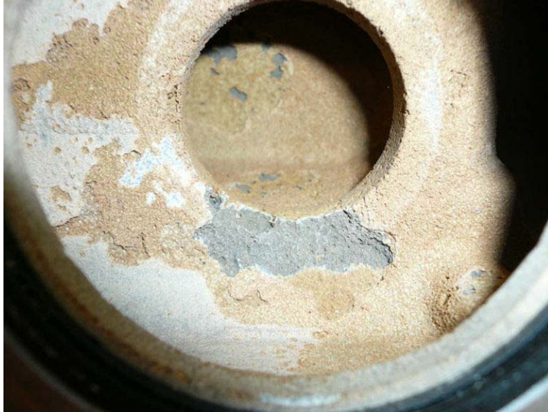
A 11 Aluminium thermostat cover, corroded
